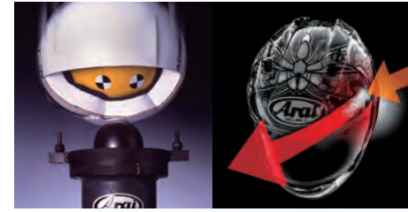
All helmets protect the rider's head through both glancing off and energy absorption.
